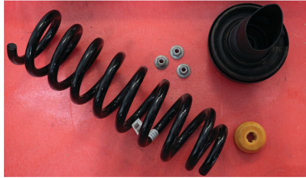
Fig. 10: OEM spring and associated hardware.
