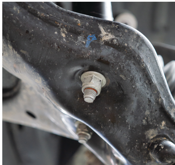
Fig. 7: Remove the bar-pin bolts.
