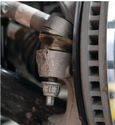
Fig. 16: Tie rod end link.
