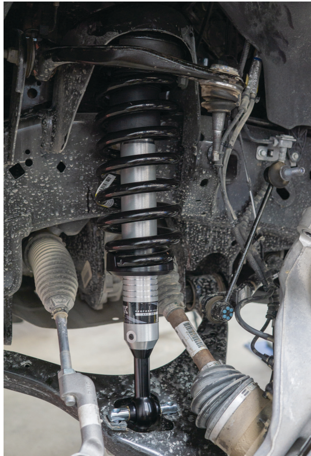
Fig. 14: Install the coil-over.
