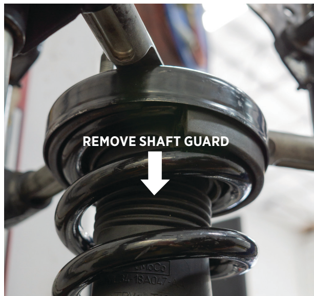
Fig. 12: OEM spring and top hat orientation.
