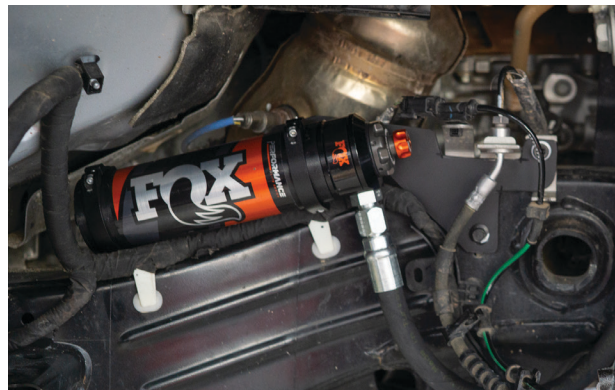
Fig. 16b: Mounted reservoir.
