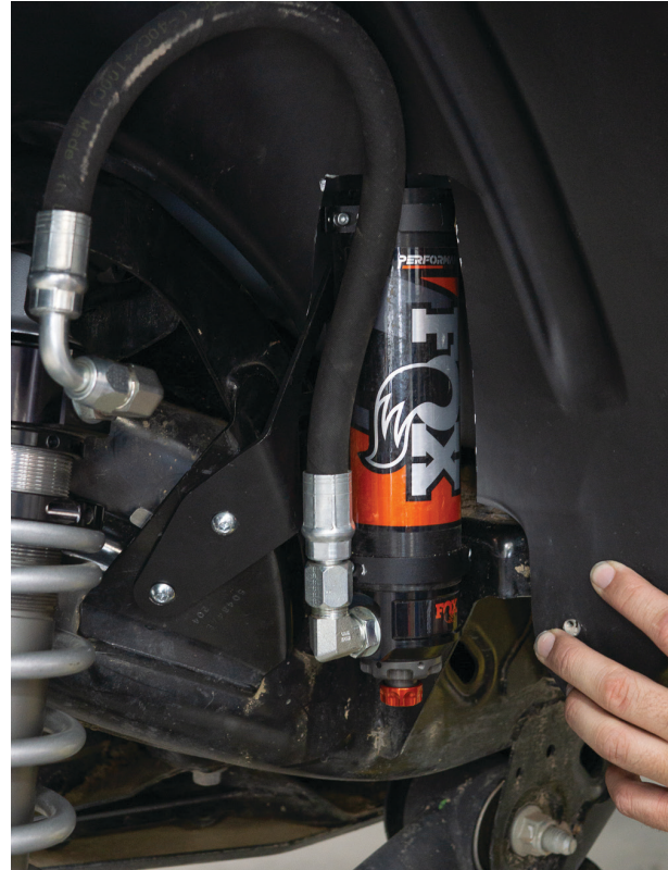
Fig. 37: Cut fender liner.
