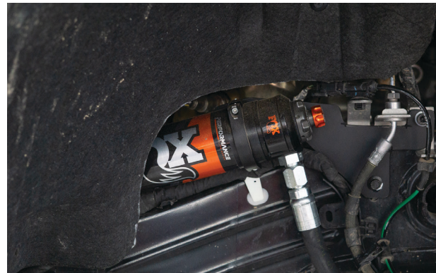
Fig. 23: Cut fender liner.
