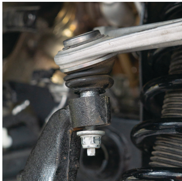
Fig. 8: Separate the UCA from the upright.
