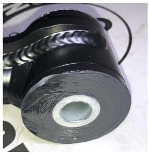
M. Install the 4 provided 90° zerk fittings into the threaded holes on the top of each bushing eye-ring ensuring they face outboard for easy access during service.
