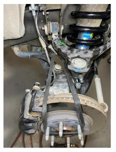
F. Using a 15mm wrench and socket, remove the sway bar link and lower shock bolts.
