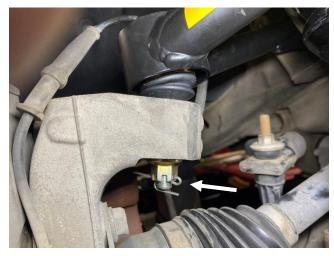
Using the supplied hose clamp, screw, locknut, and 2 washers, secure the ABS line to the tab on the UCA as shown below. Using a 3/8 wrench and 1/8" allen, tighten the screw and nut, then verify ABS line has adequate slack to accommodate steering and suspension motion.
