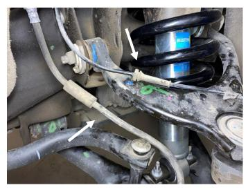
D. Using a 10mm socket, remove the ABS bracket from the top of the spindle and disconnect the ABS line from the plastic clip.
