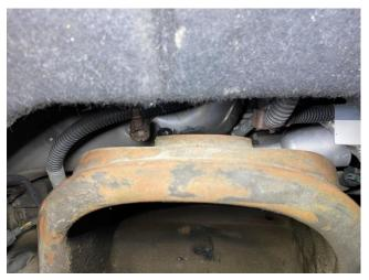
Using a 21mm wrench and socket, remove both cam bolts, then remove the OE upper control arm from the vehicle.
