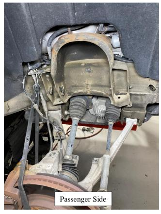
The upper control arm droop limiting bracket will need to be removed from the frame on both sides. Start by marking the cut line at the welds on both sides of the droop limiter as shown below. Then using a cut-off wheel, carefully cut the tab off of the frame.
