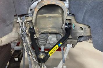
O. Reinstall the shock and spring assembly. Secure 3 top mount nuts using an 18mm wrench and lower mount using 15mm wrench and socket. Reattach the wiring harness clips to the top mount studs. Then reinstall the stabilizer link using a 15mm wrench and socket. Torque all hardware to OE specifications according to the manufacturer service manual.
