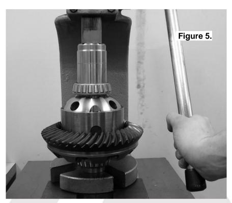
Invert the *Air Locker* and press the bearing cone which was supplied with the *Air Locker* kit onto the bearing journal on the ring gear flange side of the differential (the seal housing side) until the bearing seats firmly against the bearing journal shoulder.
