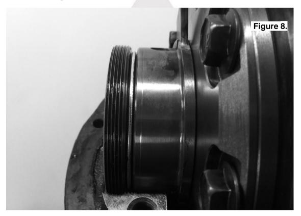
☐ Insert the bearing cap bolts and hand tighten.
