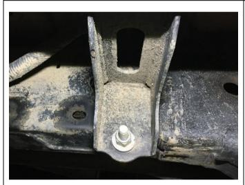
12. Using 2x M12 nyloc nuts and washers, fasten the slider to the U-bolt Leave loose for now.
