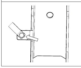
13. Using P-Clip provided, attach the wiring harness with an M6x25 bolt and washer to the rear mount cage nut, so that the harness will not rub.
