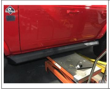
9. Using a lift table or a friend, lift the LH slider into position and fasten the two body mount nuts onto the studs. Leave loose for now.
