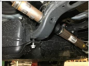
16. Moving to the RHS, if the vehicle is equipped with a gas tank skid, loosen all the bolts holding it on. Remove the three outboard bolts on the frame while installing the slider, these will be reinstalled later.
