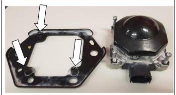
3. Gently pry the radar free of the plastic clips in the mounting plate. Remove the 3 plastic clips from the plate and put aside for later use.
