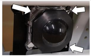
7. Carefully push the radar sensor into the plastic clips ensuring that they all clip in firmly.
