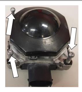
Remove the 3 Torx drive ball screws from the radar and refit from the back side .Leave approx. 3 turns of thread visible on the screw. **Do not** bottoming out the bolt into the plastic thread.
