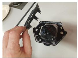
2. Remove the rubber seal from the front by unclipping the 4 side tabs.
