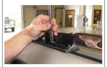
2. Carefully remove the factory bolts, metal brackets and bars.
