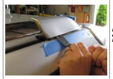
Carefully remove the plastic roof bar covers from each end of the roof bars by gently prying off, see below.
