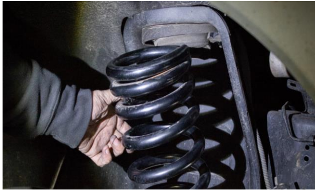
Figure 3: Front Spring Removal
