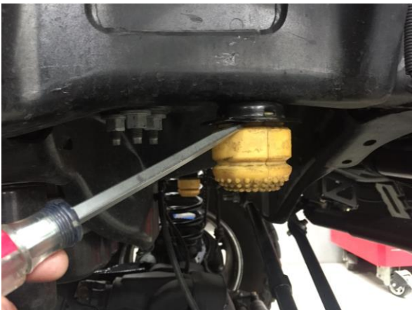
Figure 4: Bump Stop Spacer Removal
