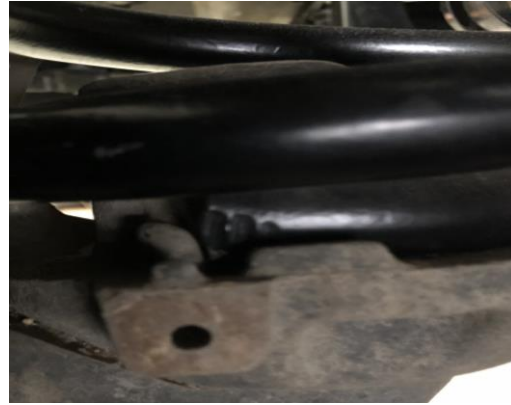
Figure 9: Bottom Spring Pigtail Installation
