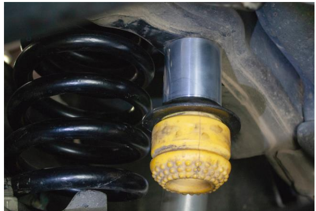
Figure 7: Assembled Bump Stop Installation
