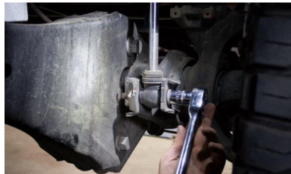
Figure 2: Front Shock Lower Bolt Removal
