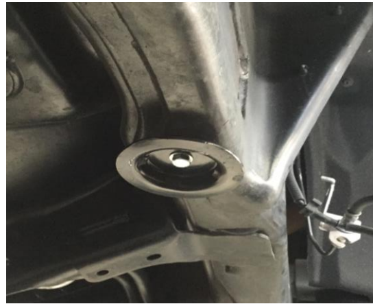
Figure 5: Bump Stop Mount Removal
