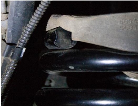
Figure 8: Top Spring Pigtail Installation
