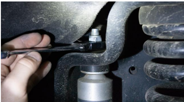
Figure 1: Front Shock Upper Nut Removal
