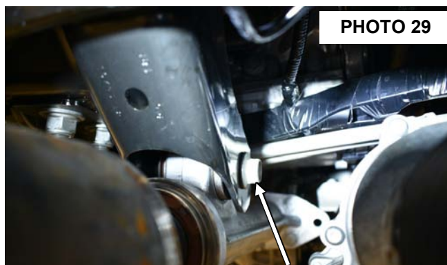
Remove the pass diff bolt.
