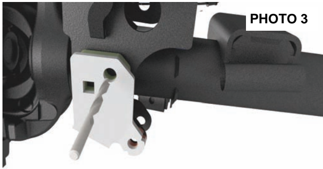
Drill using 19/32" drill.
