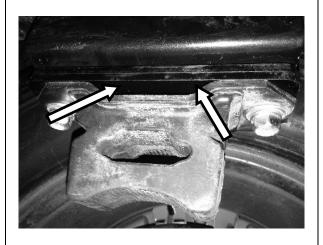
2. INSERT THE BUMP SPACER PLATE UNDERNEATH THE BUMPSTOP AND REATTACH THE RUBBER BUMP STOP USING THE ORIGNAL BOLTS. TORQUE BOLTS TO MANUFACTURES SPECIFICATIONS.
