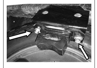
1. LOCATE AND REMOVE THE TWO M12 BOLTS WHICH LOCATE THE BUMPSTOP ON THE VEHICLE.
