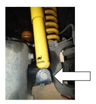
Where radius arm mounts to axle, loosen but <u>do not</u> remove the two M18 bolts.
