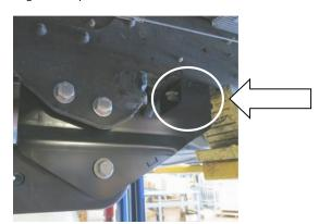
12. Tighten supplied 2 x M18 Bolts and Nyloc nuts on radius arm bracket. Torque to 350Nm (260 lbf.ft)
