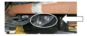
10. Insert M12 x 60mm to fix rear end of OME drop bracket to chassis and Tighten. Torque to  $80\mathrm{Nm}$
