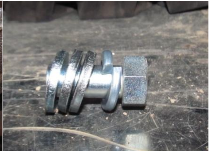
Figure 2: washers on female bolt
