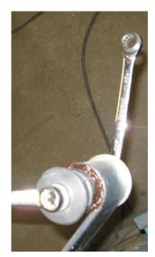
Fitting the bearing separator & puller again to push the bush in further so it is centrally located in the spring.
