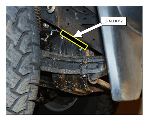
Replace the original bolts with the longer bolts supplied and tighten.
