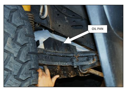
The black steel spacers (two pieces per side) are to be fitted between the oil pan and chassis on both sides.
