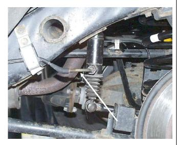
Cable must run at 90° to cylinder. Adjust if required.
