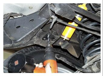
Drill two 8mm holes where previously marked.
