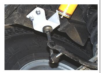
Bolt the extension bracket in position using the supplied bolts.
