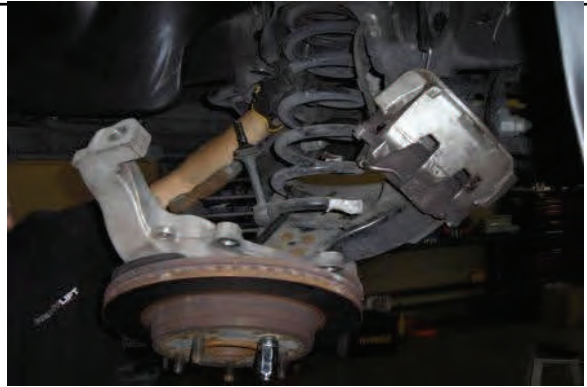
Slowly lower suspension and remove coil spring.
