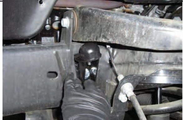
Note: pass/dr side brackets are specific. Tighten once aligned
