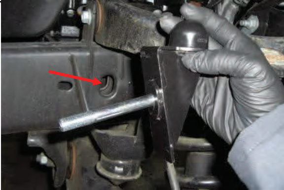
Attach new bump stop and bracket to frame as pictured
