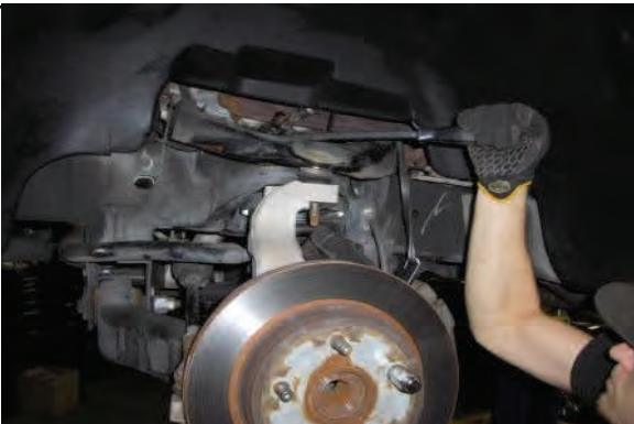
Carefully lift suspension enough to engage upper ball joint.
