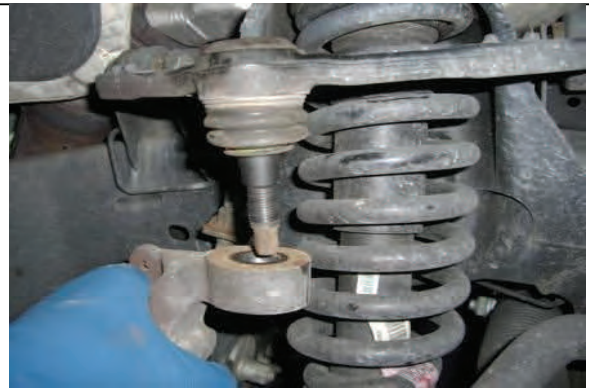
Carefully strike spindle with hammer to break loose, separate
