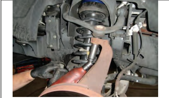
Tighten upper ball joint and torque to spec.
