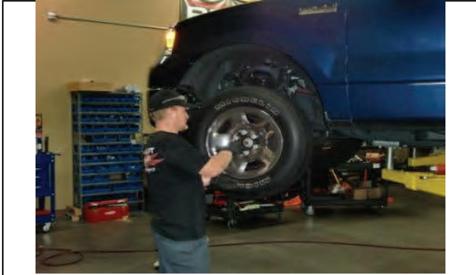
Install wheels/tires torque to spec., measure and align
