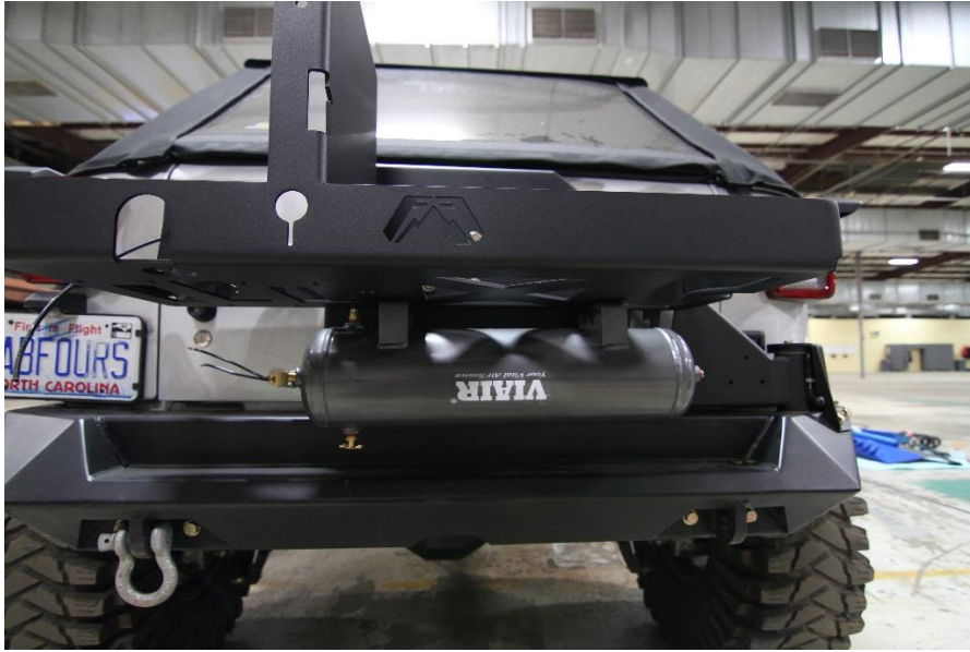
Figure 1: Air Tank Installation
