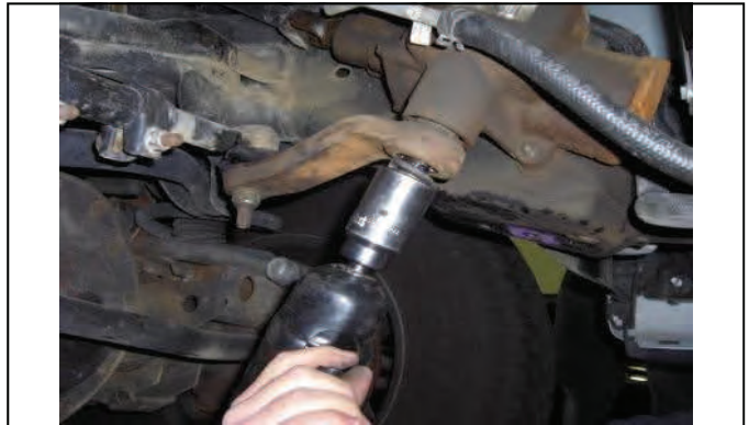
Remove pitman arm mounting nut
