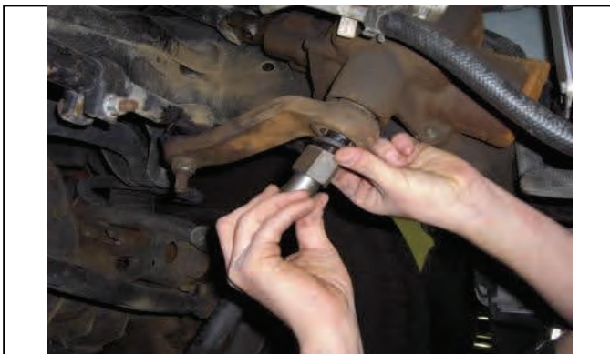
Place extension onto sector shaft with lock washer as shown
