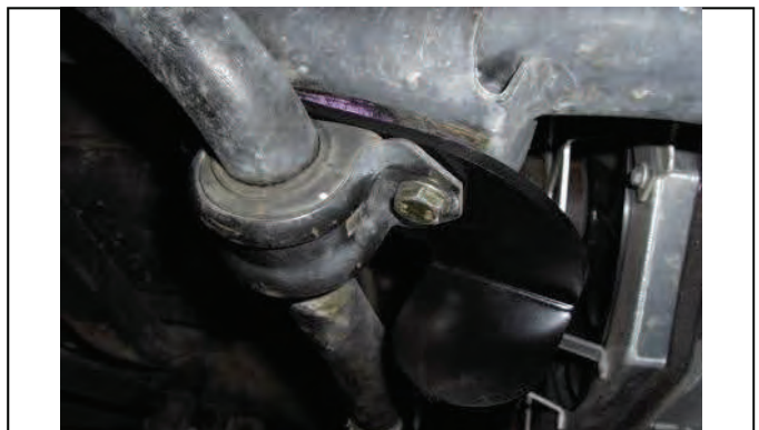
Start new hardware to reattach sway bar through bracket
