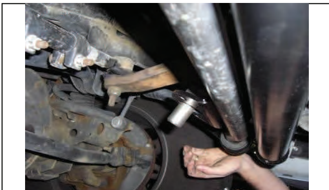
Place new stabilizer bar into position and raise sway bar
