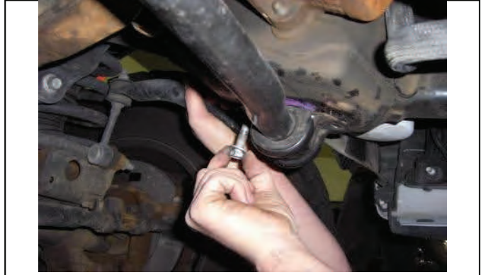
Remove sway bar mounting hardware at frame
