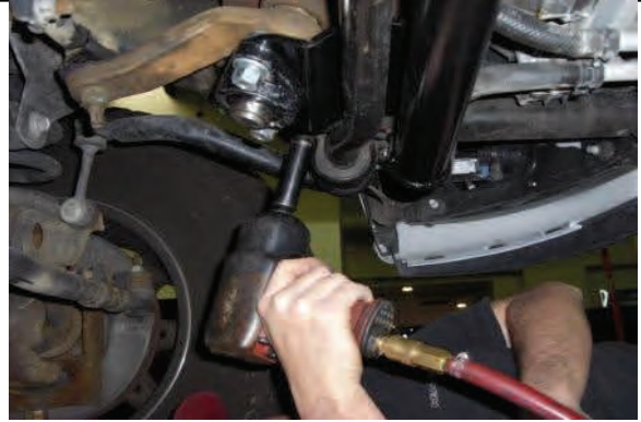
Tighten bearing and then sway bar hardware
