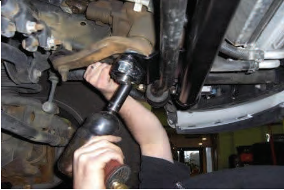
Attach locator bearing over sector shaft extension
