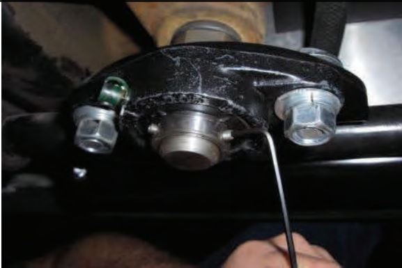
Attach bearing retainer and tighten set screws
