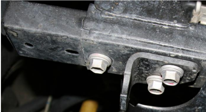
Figure 9 & 10 – Bumper beam extension and tow eye removal
