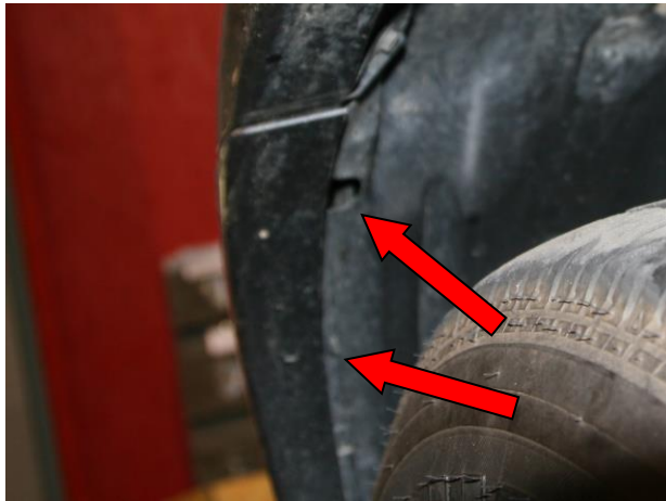
Figure 3 – Fenderwell fastener removal
