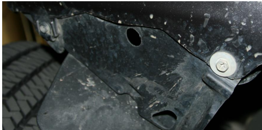
Figure 4 – OEM bumper cover screw removal
