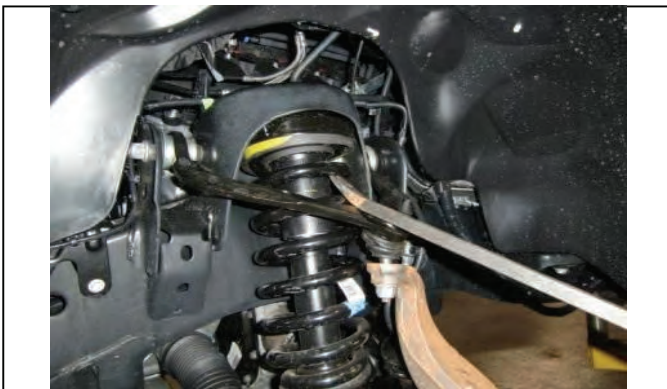
Raise suspension and reattach upper ball joint
