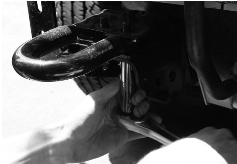
Figure 3 - Tow Hook Removal
