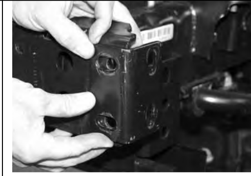
Fig 2 Note the orientation of the bolt holes
