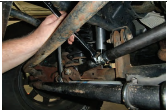
Adjust track bar to center axle and tighten jam nuts.
