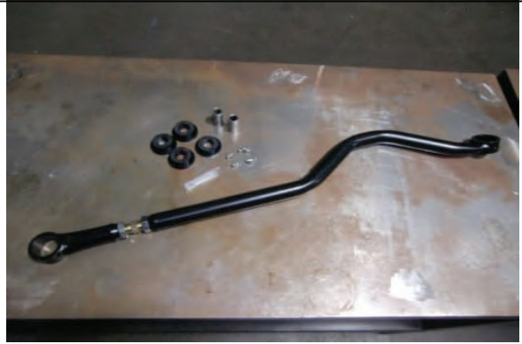
Assemble front track bar bushings, sleeves and zerk fittings
