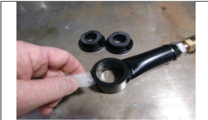
Use assembly lube to fit bushings and sleeves.
