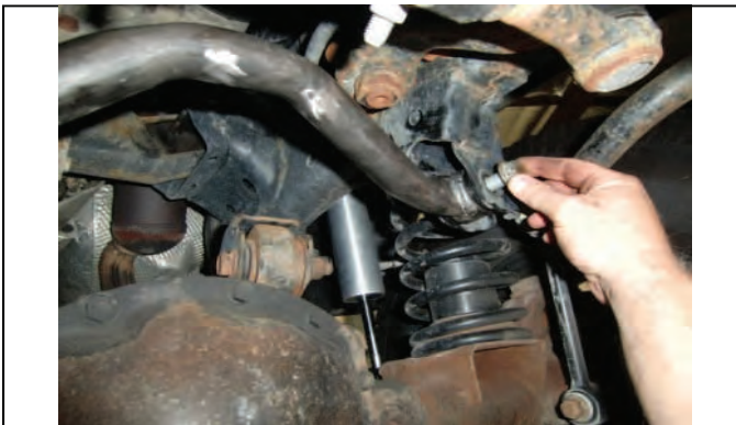
Reinstall adjustable track bar in reverse order of removal
