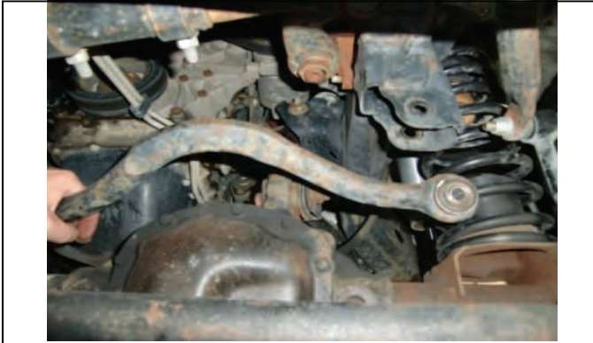
Remove track bar from vehicle
