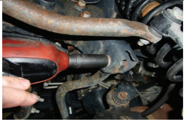
Remove hardware at the frame as well.
