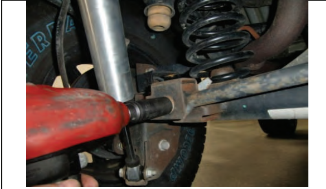
Remove rear track bar bolt at axle.
