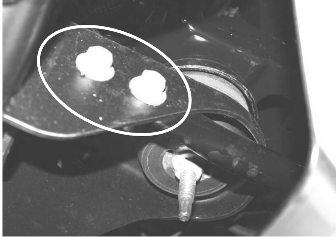
Figure 4 – Outer Bumper Support Screws
