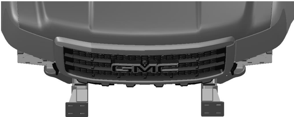
Figure 11 - Intermediate Bracket Orientation
