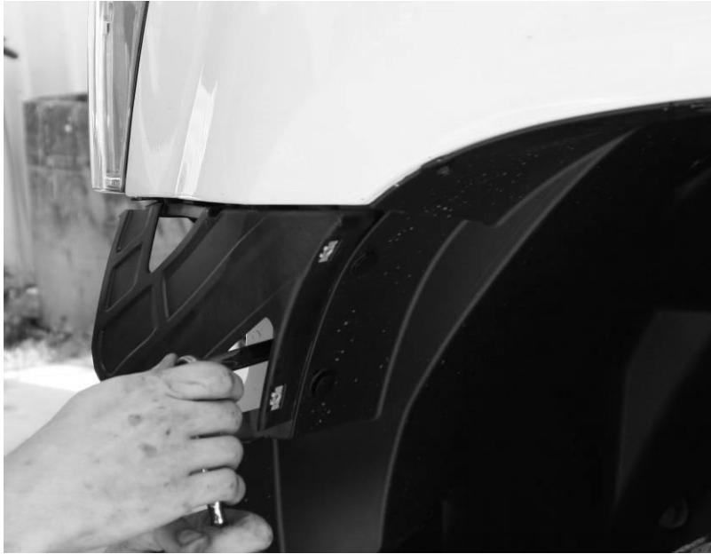
Figure 6 - Support Bracket Removal
