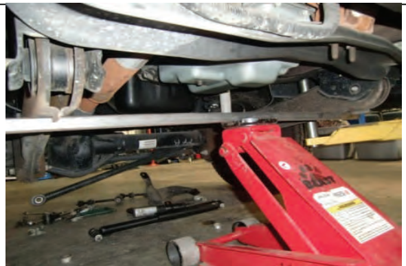
Block front wheels, use a jack w/crossbar to support arms
