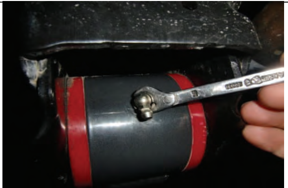
Install provided zerk fittings and reconnect ABS/vacuum lines
