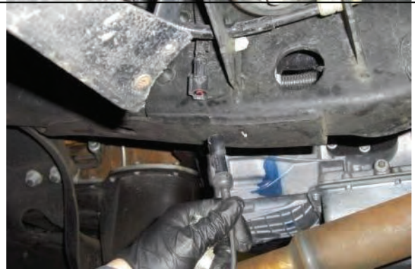
Disconnect ABS line at plug above radius arms
