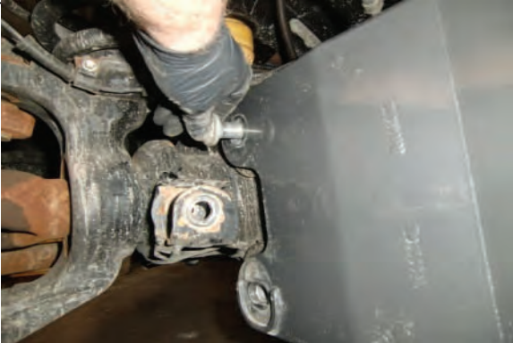
Install new assembled radius arm w/ OE bolts at top
