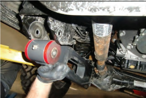
Raise radius arm into frame, attach w/ OE hardware
