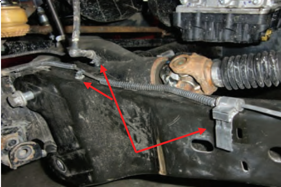
Remove all wiring clips from radius arms
