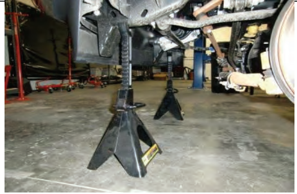
Support weight of the vehicle by frame. Min. 3 ton jacks
