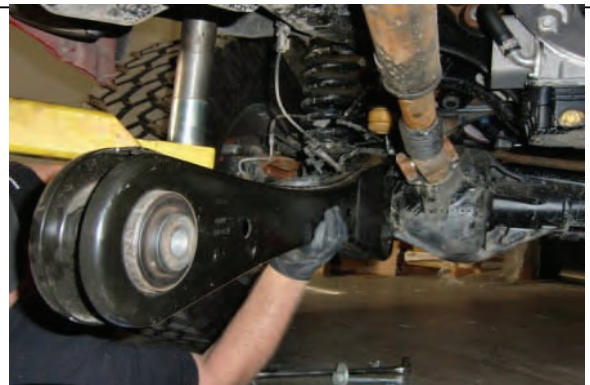
Lower slowly & remove front radius arm hardware and arms
