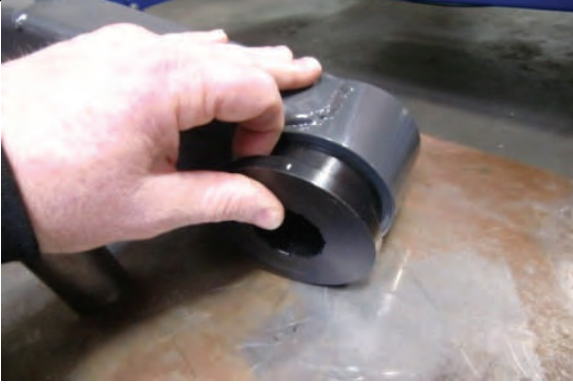
Use assembly lube to install urethane bushings
