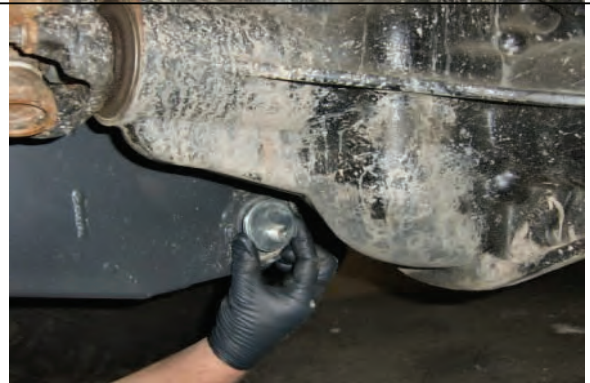
Install new offset cams/bolts/nuts into front lower mount
