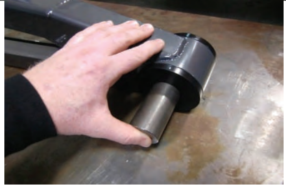
Lube pivot pin and install into bushings
