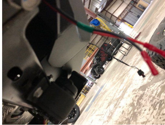
Figure 4. Inserting the OEM license plate light into the M4550 license plate bracket.
