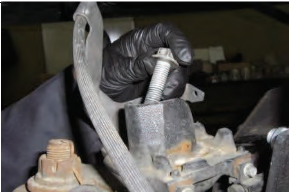
Remove bolt from middle of spring perch
