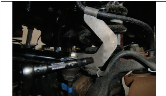
Disconnect brake line support bracket
