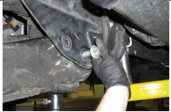
Support radius arm and remove attachment bolts
