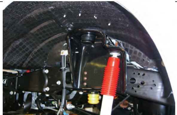
Carefully lower axle and remove coil spring
