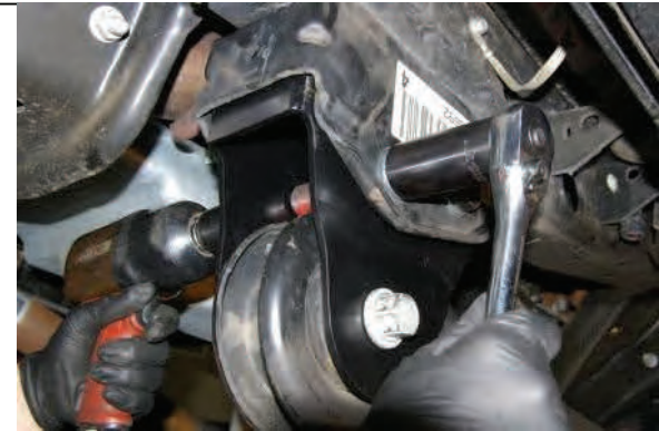
Tighten hardware and leave OE bolt loose until on ground.
