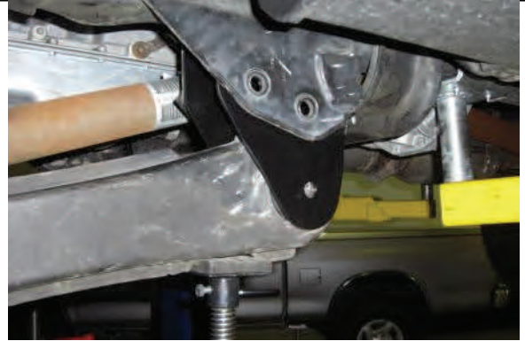
Align bracket with holes in frame and raise arm into bracket.
