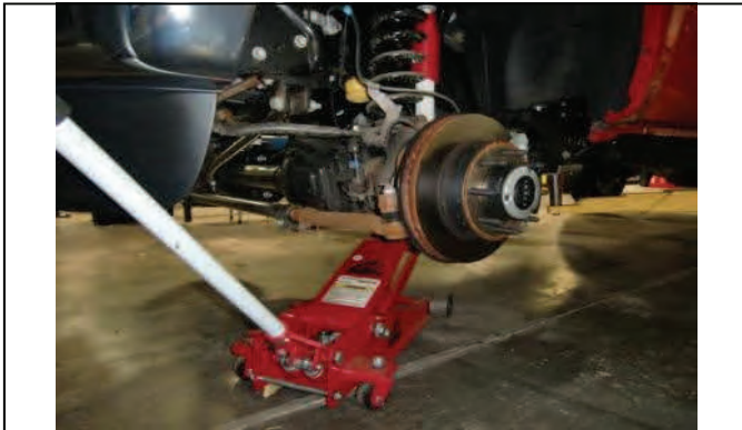
Support front axle with floor jack(s).
