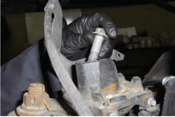
Remove bolt from middle of spring perch
