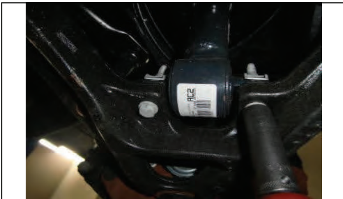
Remove lower strut mounting bolts
