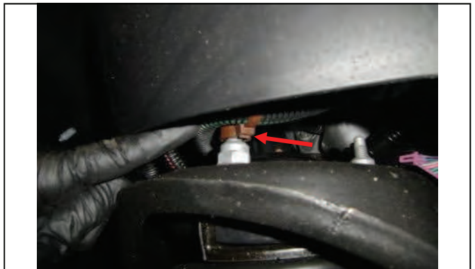
Unclip upper strut ABS clips on mounting nuts
