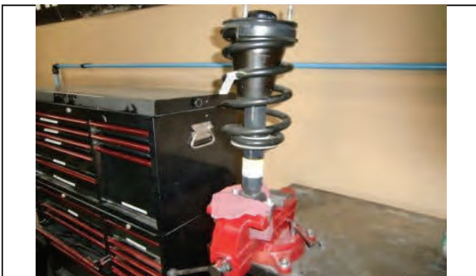
Place strut in vise or spring proper compressor
