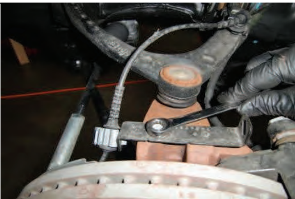
Disconnect ABS bracket on spindle
