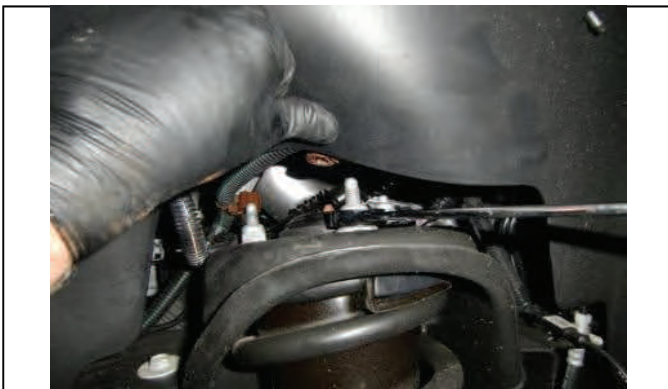
Remove upper strut mounting nuts
