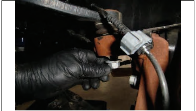
Now remove nut from ball joint
