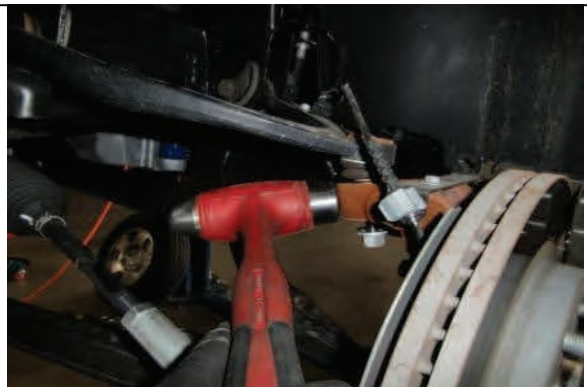
Strike spindle with hammer to loosen ball joint
