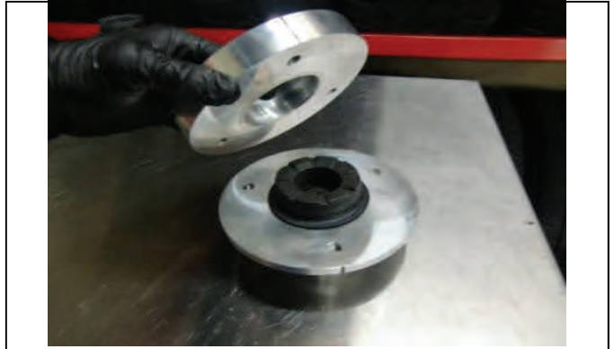
Place OE strut bushing between two halves
