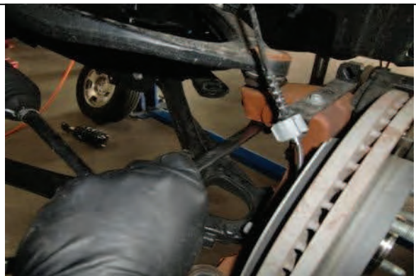
Loosen upper ball joint nut
