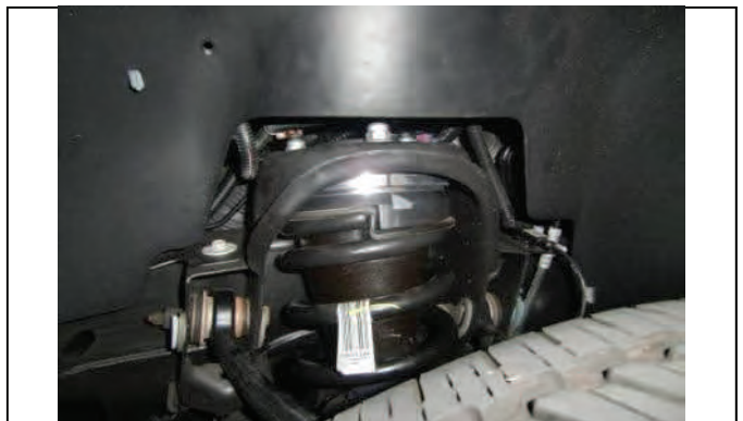
Install strut assembly w/ new nuts on top, OE in lower
