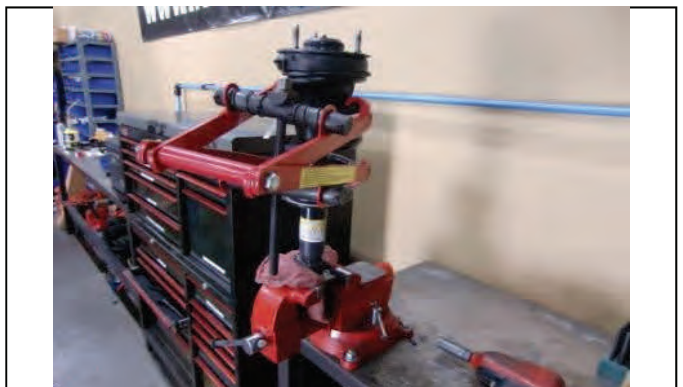
Use spring compressor to relieve tension for disassembly
