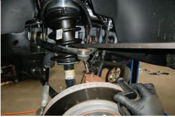
Raise suspension to reconnect ball joint to spindle
