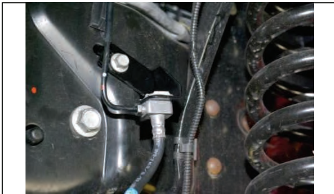
Reinstall block into bracket with retaining clip.
