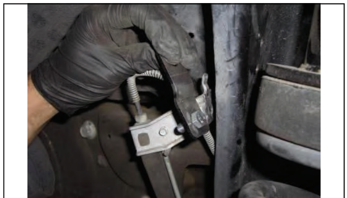
Install drop bracket and attach to frame with OE hardware.
