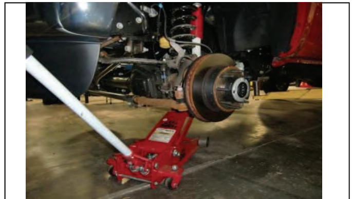
Support front axle with floor jack(s).
