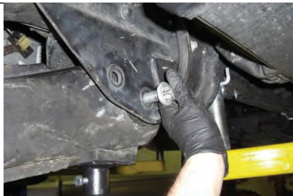
Support radius arm and remove attachment bolts
