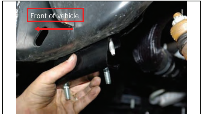
Install provided drop brackets to frame with OE hardware.
