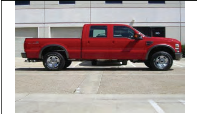
Place vehicle on level ground and measure ride height.
