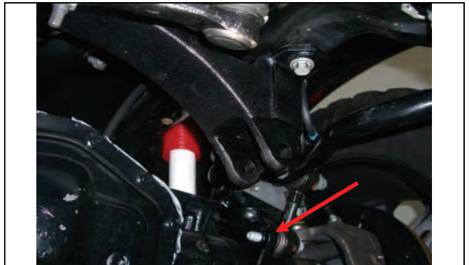
(05-10) Re-attach and tighten sway bar end links.
