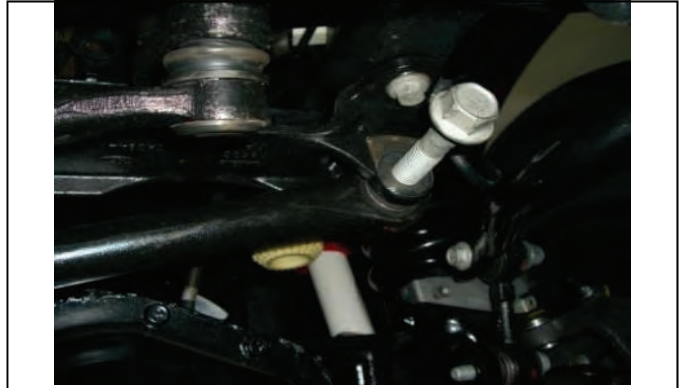
Remove upper trac bar hardware and disconnect at frame.
