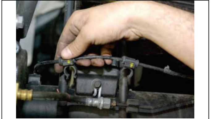
Vehicles with ABS/TC remove clips from U-bolts.
