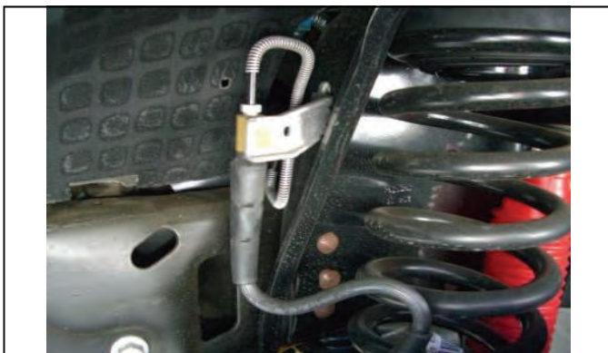
(05-07) models remove brake line brackets at the frame
