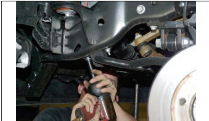
(11-up next 3 steps) Disconnect sway bar at frame and lower
