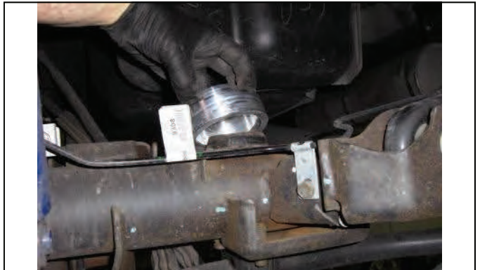
Place ReadyLIFT spacer on axle mount
