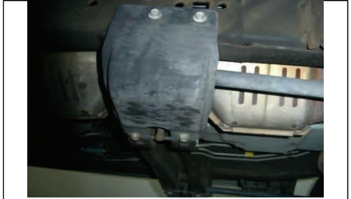
Locate cross member cover and remove bolts
