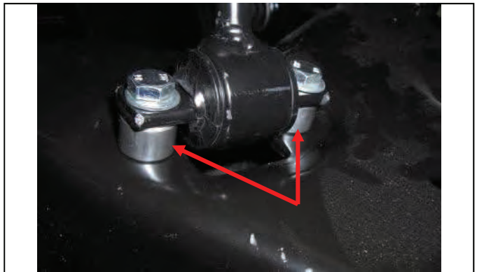
Install shock spacers as shown
