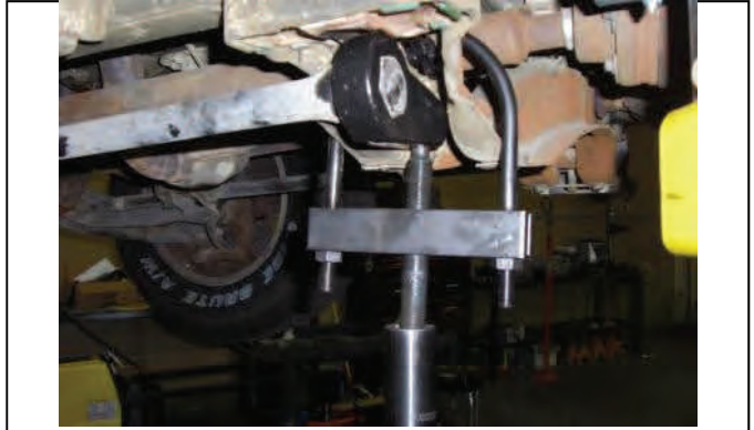
Adjust torsion key tool enough to replace keeper block
