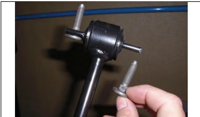
Remove both bolts and use new provided hardware
