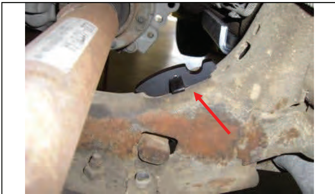
Place torsion bar unloading tool adapter above cross member
