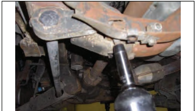
Remove torsion key adjuster bolt
