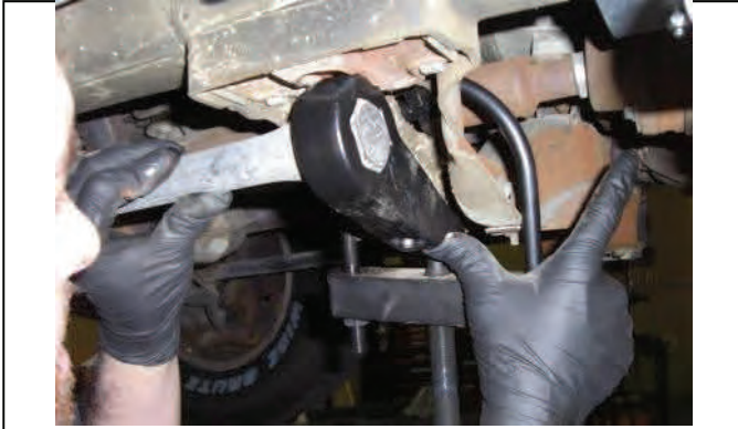
Install new torsion key and reload tool
