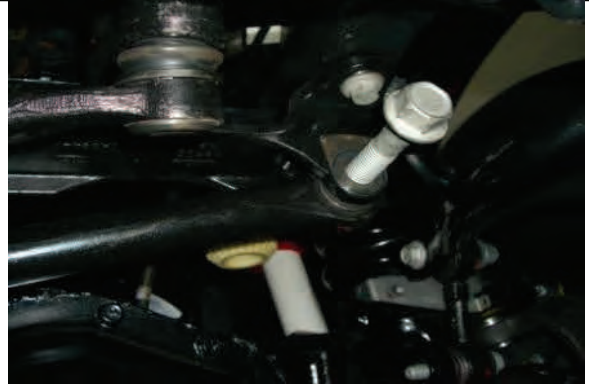
Remove upper trac bar hardware and disconnect at frame.
