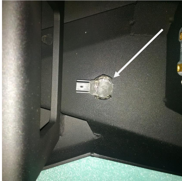
Figure 3 Inner passenger side sensor orientation
