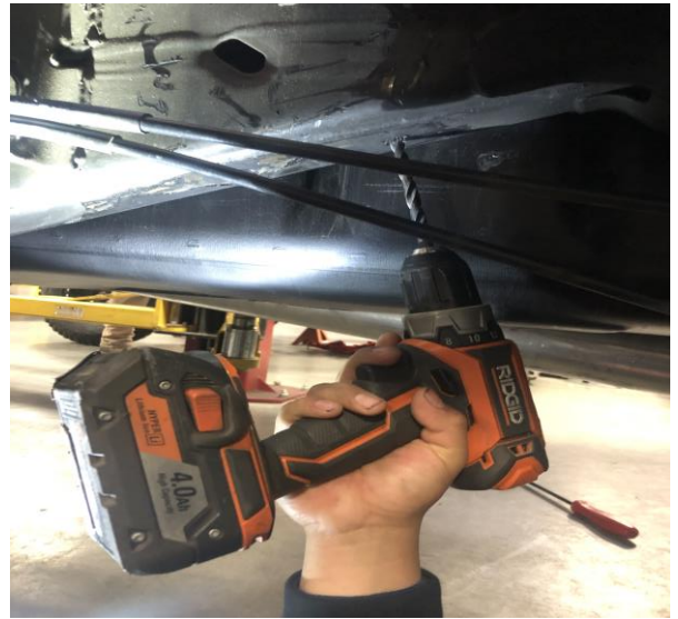
Figure 7: Drill Frame Mount Holes
