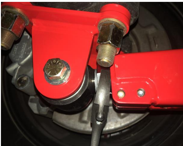
Figure 36: Traction Bar Length Adjustment
