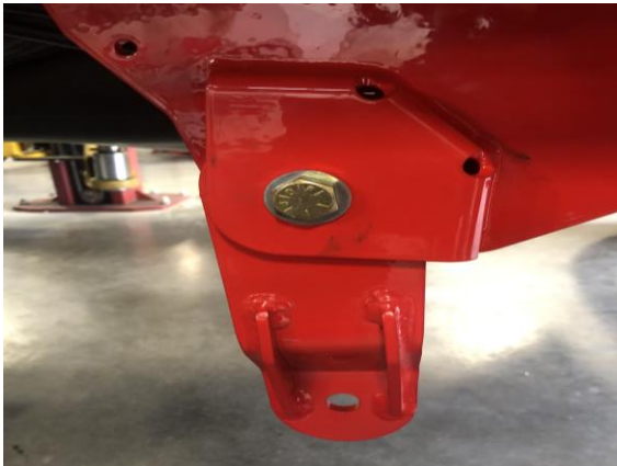
Figure 19: Assemble Shackles to Frame Mount
