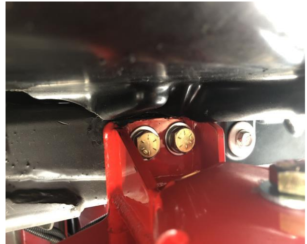
Figure 13: Fuel Tank Shield Trimmed
