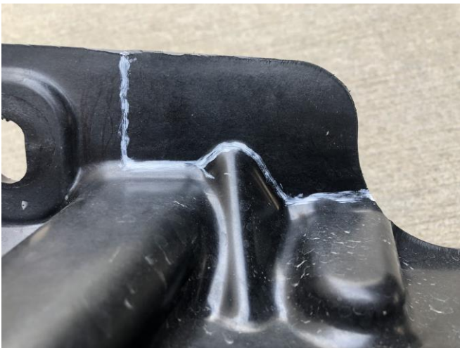
Figure 12: Fuel Tank Shield Trim
