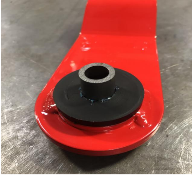
Figure 17: Install Shackle Crush Sleeves
