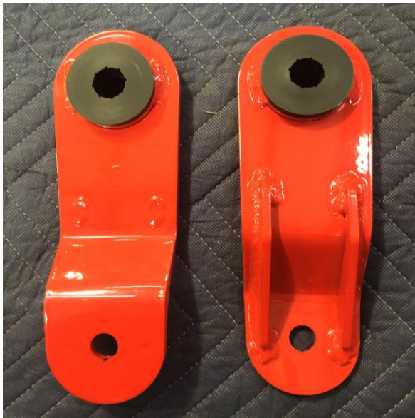
Figure 15: Install Shackle Bushings
