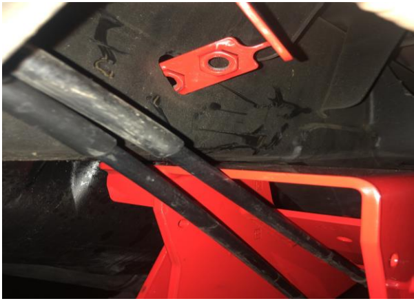
Figure 10: Insert Nut Plate
