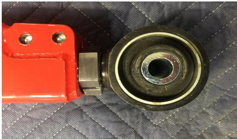
Figure 33: Traction Bar Rod End
