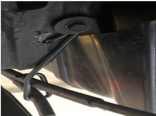
Figure 1: Remove Brake Cable Bracket
