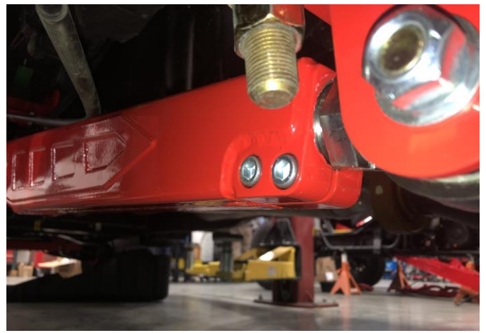
Figure 37: Adjuster Nut Clamp
