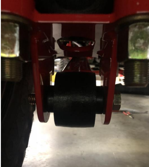
Figure 34: Traction Bar Rod End / Rear Axle Pivot
