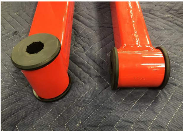
Figure 28: Traction Bar Bushings Installed
