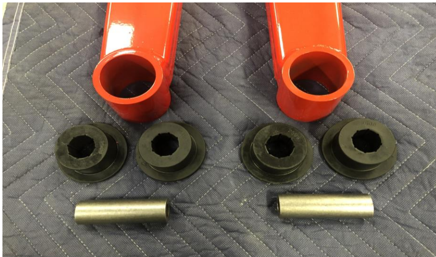
Figure 27: Traction Bar Bushing Parts
