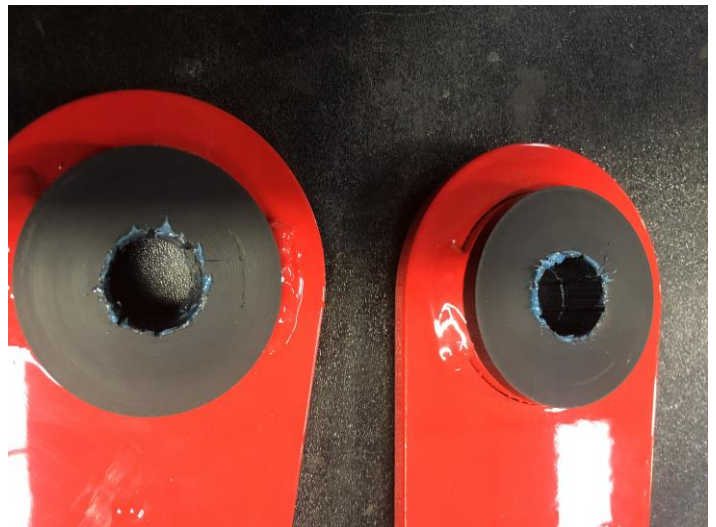
Figure 16: Grease Shackle Bushings
