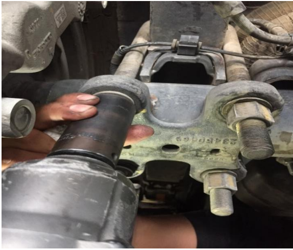
Figure 25: Remove U-Bolt Nuts
