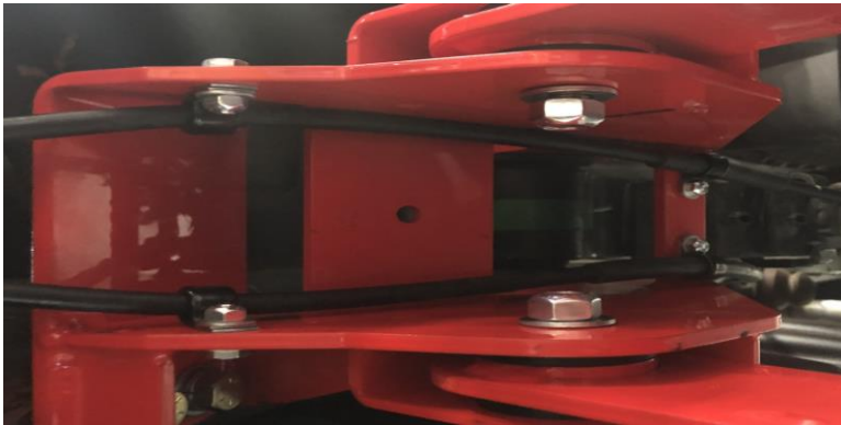
Figure 21: Route Brake Cables
