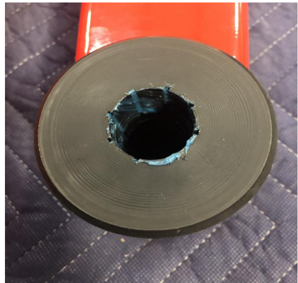
Figure 29: Traction Bar Bushings Greased
