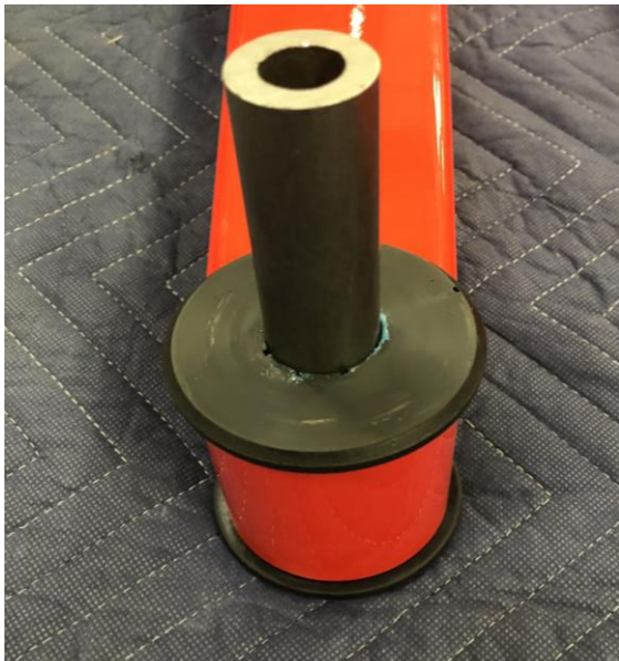
Figure 30: Traction Bar Assembled
