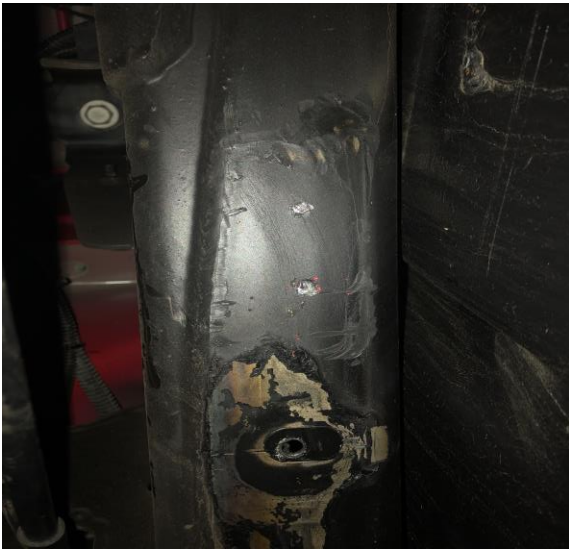
Figure 6: Frame Mount Hole Locations
