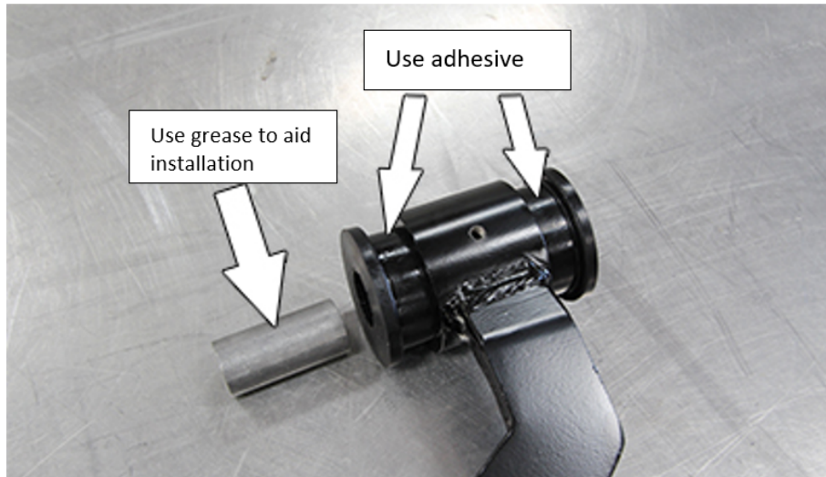
Figure 3: brushing and crush sleeve installation
