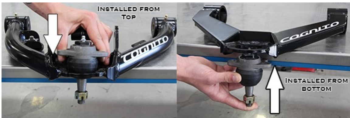
Figure 2: ball joint installation
