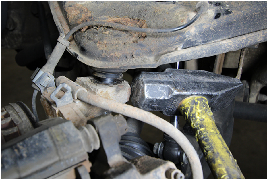
Figure 1: breaking ball joint loose from spindle
