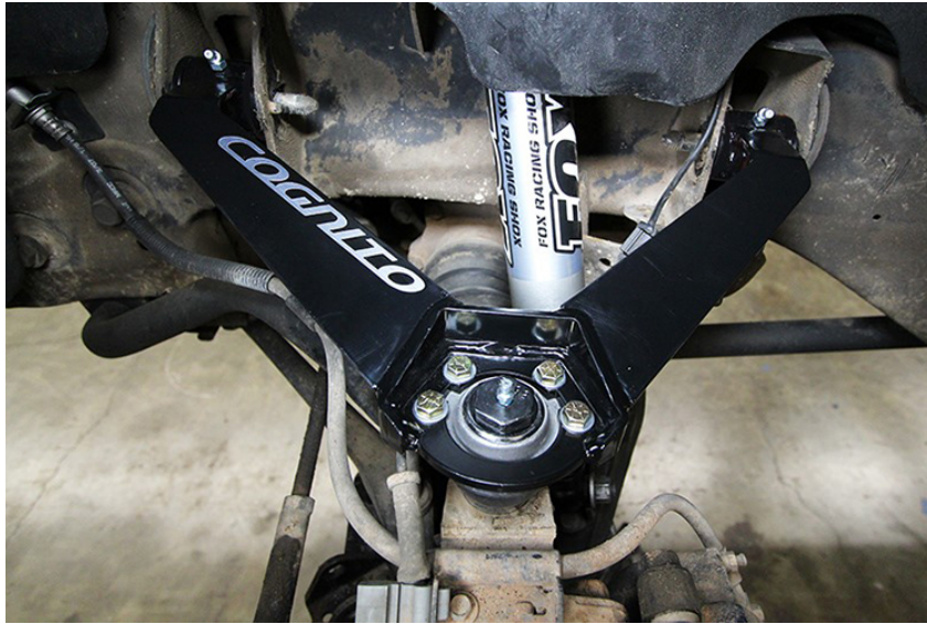
Figure 4: Driver side Cognito control arm installed
