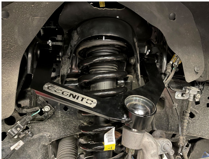
Figure 13: Cognito SM Series UCA Installation
