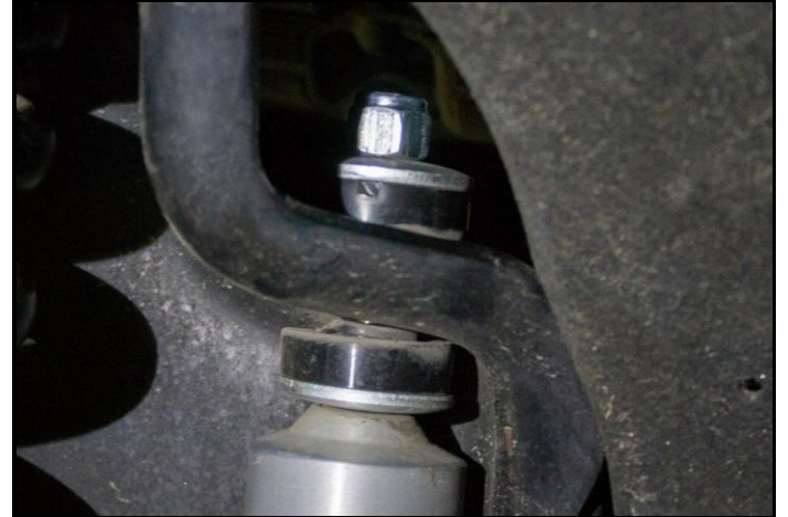
Figure 56: Top Shock Mount Installed
