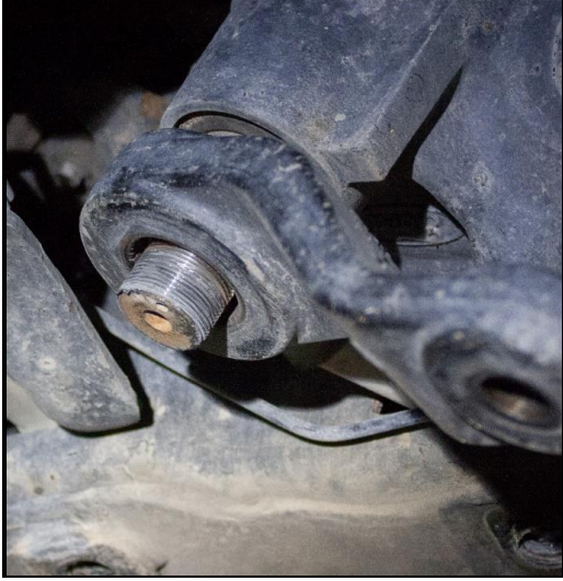
Figure 21: Steering Box Nut Removed
