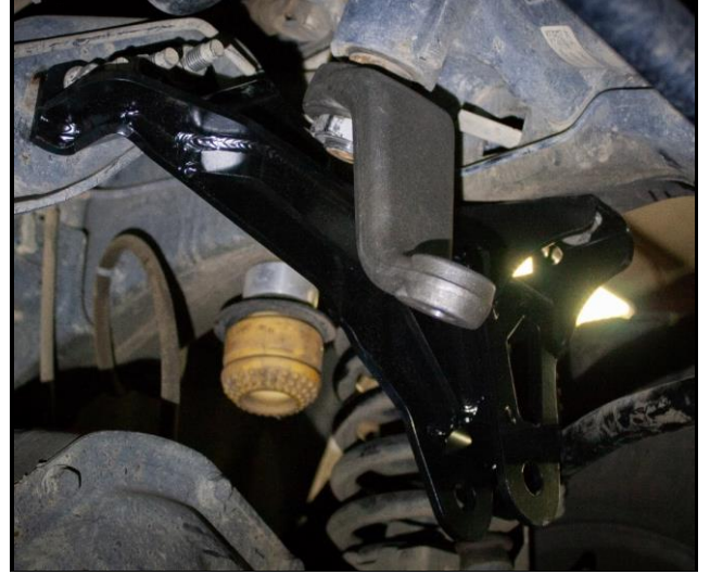
Figure 26: Cognito Track-Bar Bracket Installed
