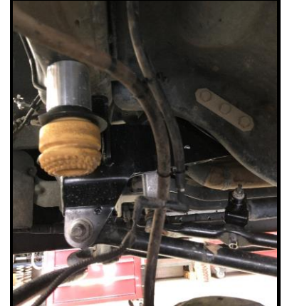
Figure 60: ABS Line Installed
