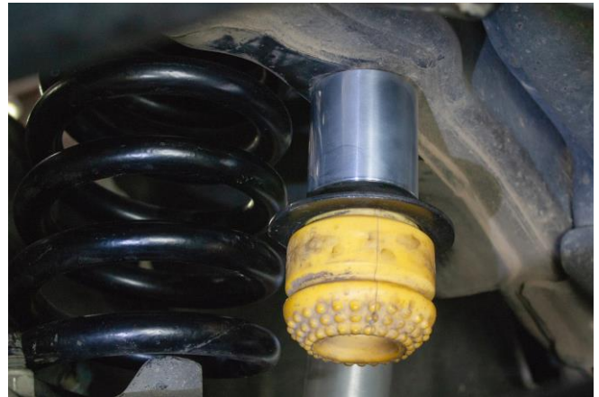
Figure 13: Bump Stop Spacer Orientation
