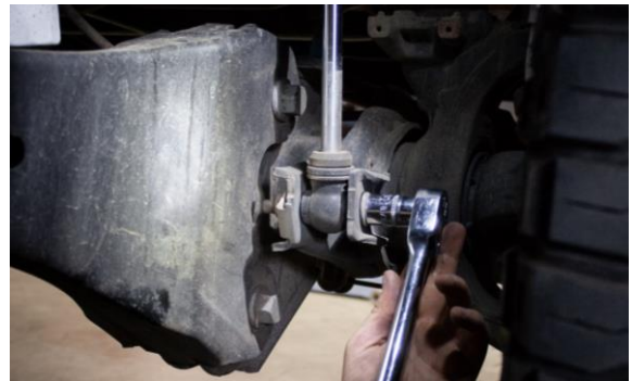
Figure 8B: Front Shock, Lower Mount
