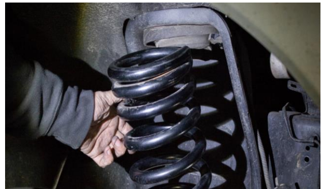
Figure 9B: Spring Removal
