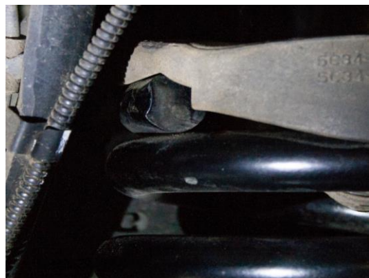
Figure 14A: Coil Spring and Isolator Orientation
