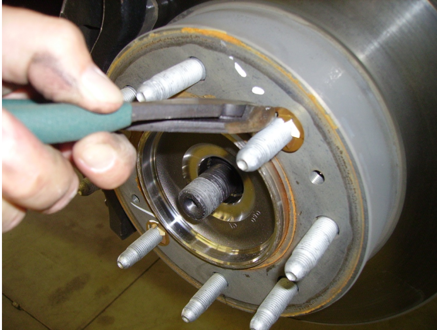
Figure 3 Remove clips from all 4 corners of vehicle. MUST DO for aftermarket wheels.
