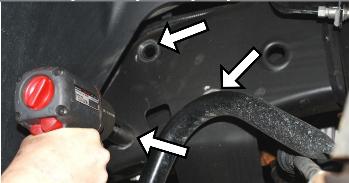
Figure 5: Removing Bolts Holding Steering Box to Frame
