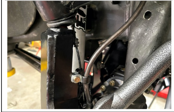
Figure 63: Passenger Side: Top Spindle Tab and P-clamps
