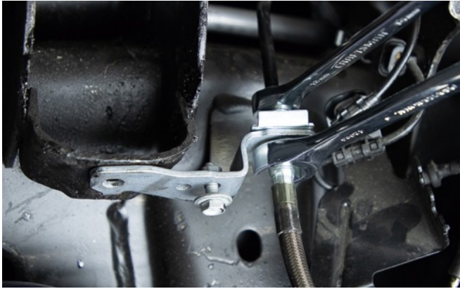
Figure 29: Cognito Extended Stainless-Steel Brake Lines
