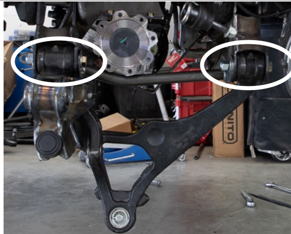
Figure 71: Lower Control Arm Bolts that do NOT get torqued at this step
