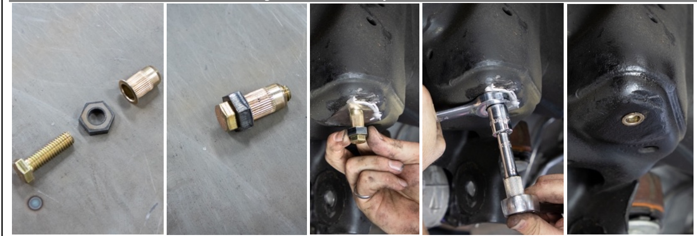
Figure 36: Install Tool for Rivet Nut
