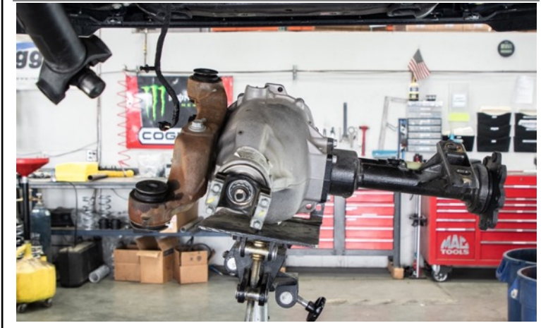
Figure 24: Lower Differential from Vehicle
