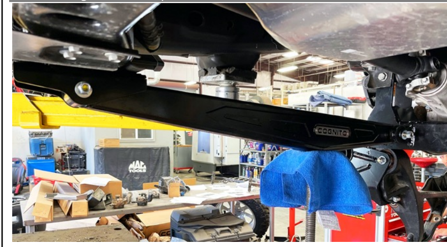
Figure 68: Compression Strut and Rear Crossmember
