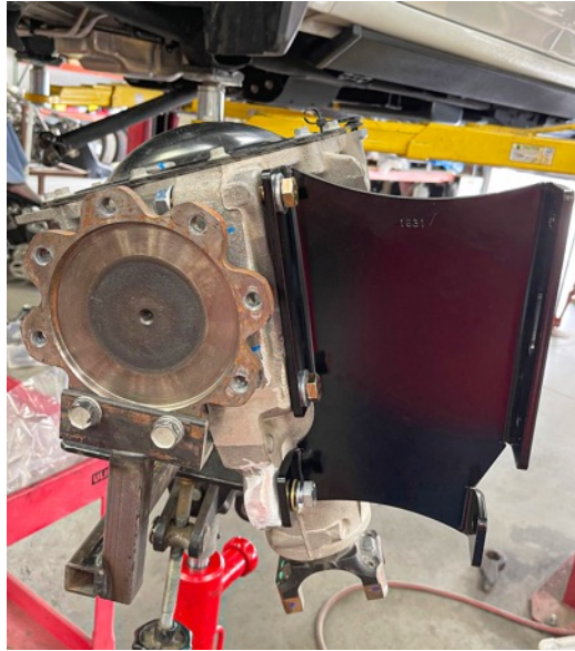
Figure 31: Mount Differential Drop Bracket Driver Side
