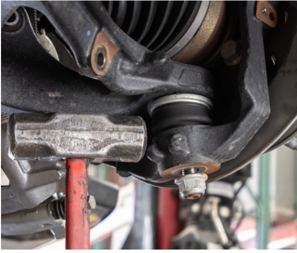
Figure 10: Loosen Lower Ball Joint
