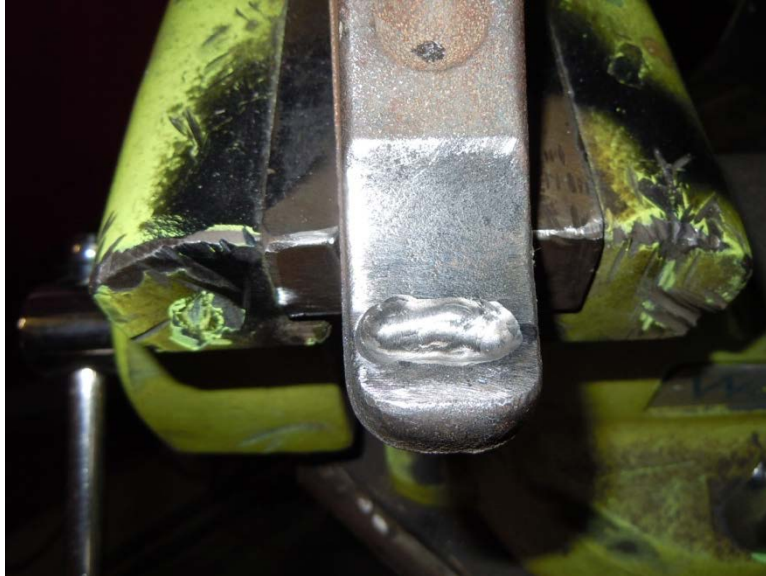
Figure 14: Use a carbide grinding bit to connect the 2 countersink spots in order to create an oval shaped pocket as shown. Now ready to install.
