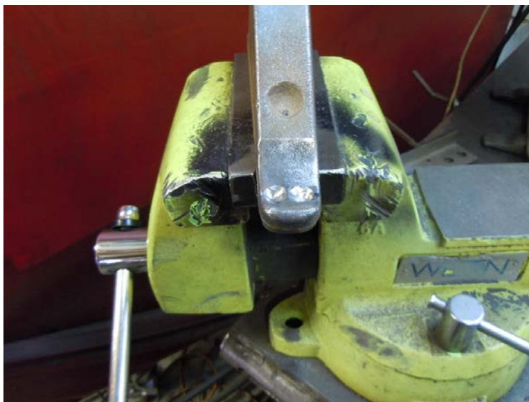
Figure 13: using a drill motor and 1/2" drill bit, drill only 1/8" deep from the tip so create 2 counter sink spots.
