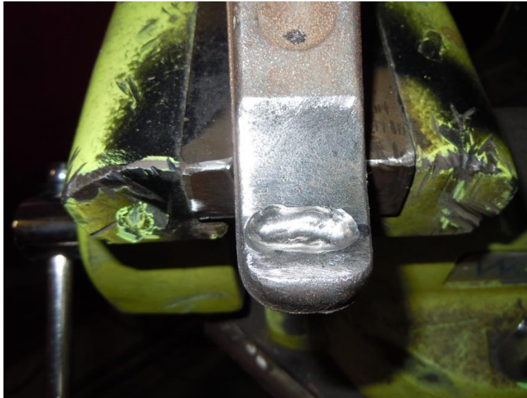
Figure 18: Use a carbide grinding bit to connect the 2 countersink spots in order to create an oval shaped pocket as shown. Now ready to install.
