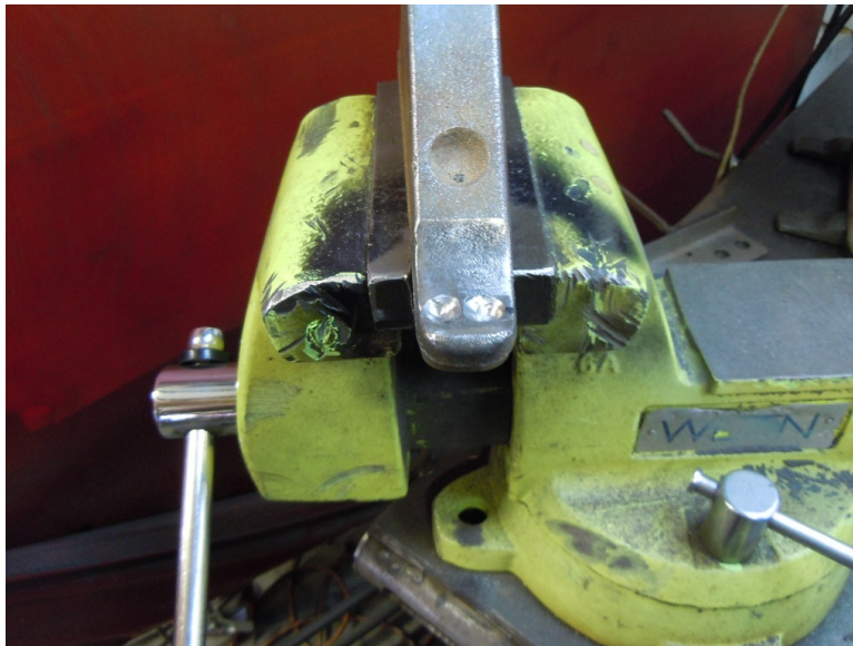
Figure 13: using a drill motor and 1/2" drill bit, drill only 1/8" deep from the tip so create 2 counter sink spots.
