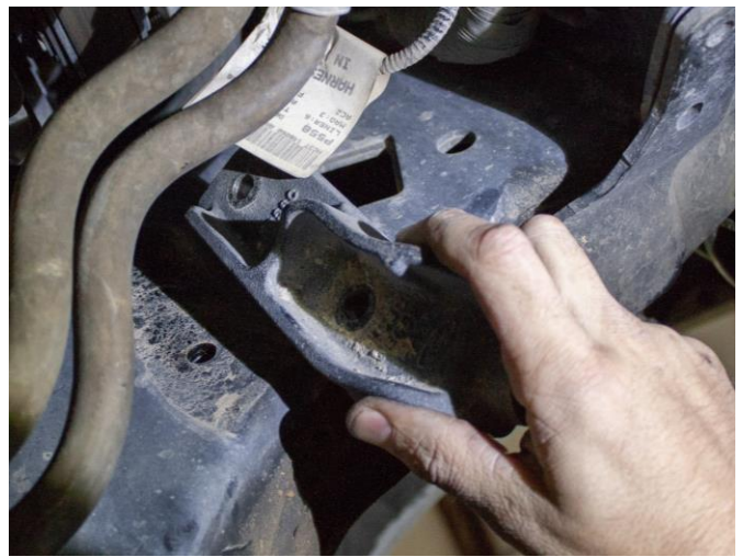
Figure 12B: Stabilizer Bracket Removed
