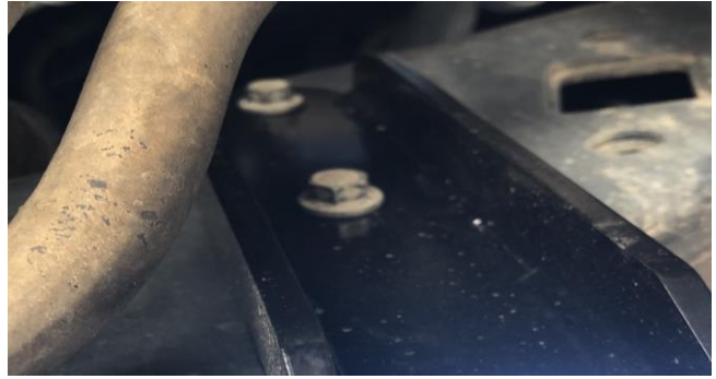
Figure 13B: Cognito Steering Stabilizer Installed
