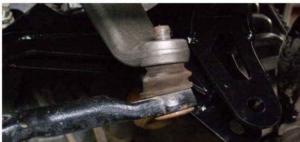
Figure 15A: Drag Link Orientation
