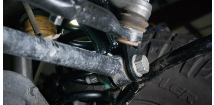
Figure 36B: Track-bar Installed
