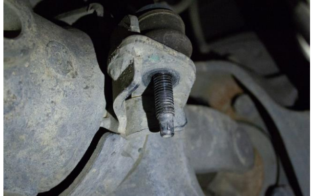
Figure 2B: OE Sway-Bar End Link, Nut Removed
