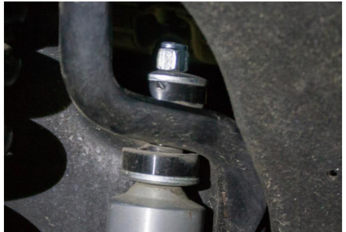
Figure 31B: Top Shock Mount Installed
