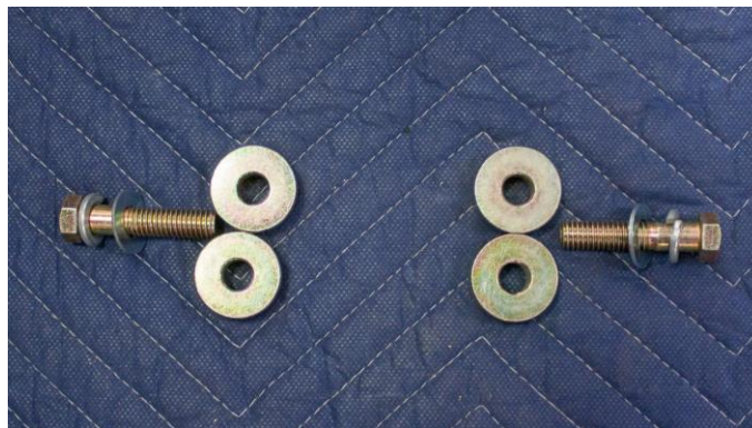
Figure 27: Center Support Bearing Spacers
