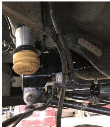
Figure 33B: ABS Line Installed
