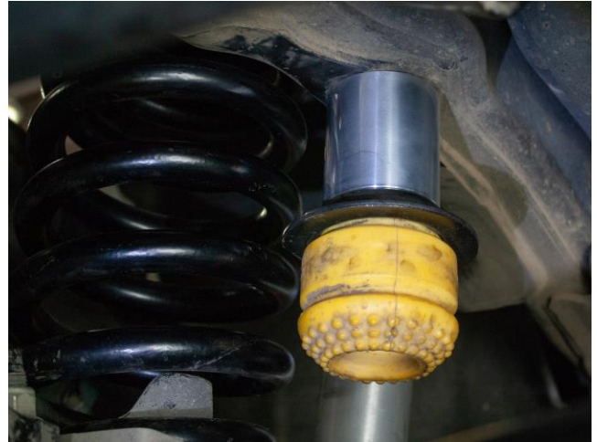
Figure 25B: Bump Stop Spacer Orientation
