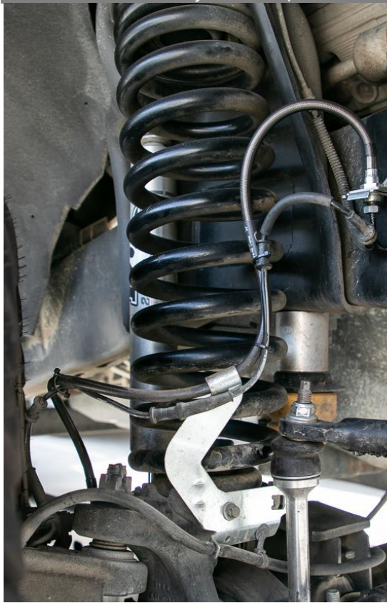
Figure 40A: Brake Line Routing (Passenger Side Shown from Front)
