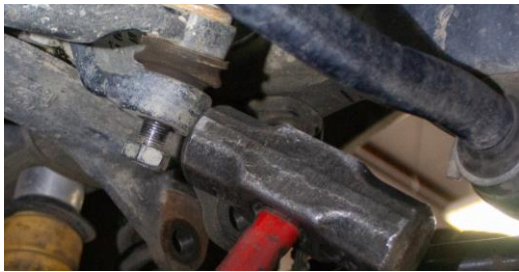
Figure 7C: Pitman Arm Taper Seat Removal
