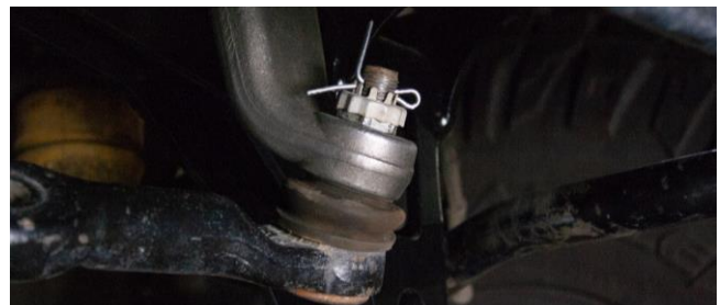
Figure 15B: Drag Link Adjuster Lock
