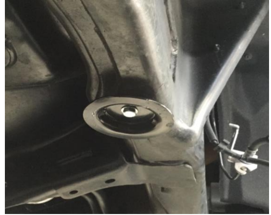
Figure 23B: FSD Bump Stop Spacer Hardware
