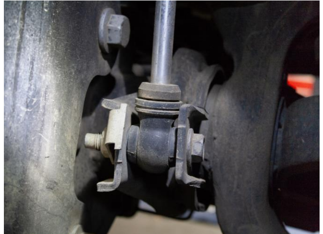
Figure 32B: Front Lower Shock Mount Installed
